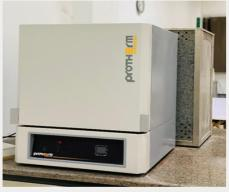
Muffle furnace (1200 C)
