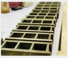
**Mortar and Concrete Molds**
