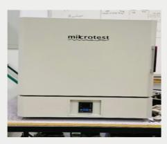
Muffle Furnace (1200 C)
