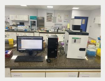
Chemiluminescence Western, Northern or Southern blot Optional applications: DNA and RNA gels and fluorescence stain imaging with UV-Pad or Blue-Pad Colorimetric stained protein gels, X-Ray film, autorads, SSCP gels, colony dish and flask imaging with WhiteLight-Pad or UV-Pad + conversion screen Fluorescence Western blot with Spectra Capsules: 365nm - 440nm - 480nm - 530nm 640nm - 680nm - 740nm - 780nm
