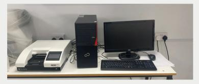
The BioTek 800 TS absorbance reader is a high-quality microplate reader for assays in 6-to 384- well formats. Applications include ELISA, protein quantification, enzyme kinetics and cell-based assays.
