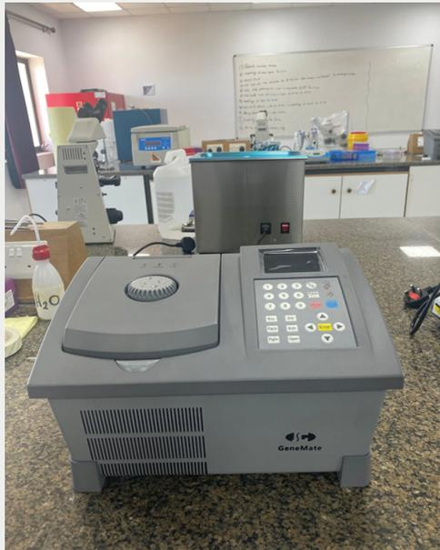
The thermal cycler (also known as a thermocycler, PCR machine or DNA amplifier) is a laboratory apparatus most commonly used to amplify segments of DNA via the polymerase chain reaction (PCR)
