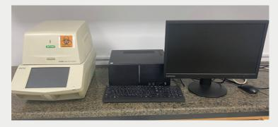
The CFX96 Touch System is a powerful, precise, and flexible real-time PCR detection system. This six-channel (five colors and one FRET channel) real-time PCR instrument combines advanced optical technology with precise temperature control to deliver sensitive, reliable detection for singlexplex or multiplex reactions.
