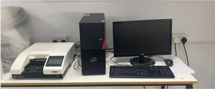
The BioTek 800 TS absorbance reader is a high-quality microplate reader for assays in 6- to 384- well formats. Applications include ELISA, protein quantification, enzyme kinetics and cell-based assays.
