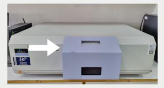
It is a molecular emission spectroscopy that analyzes fluorescence from a molecule based on its fluorescent properties (limited to fluorescent molecules). It is used in biochemical, medical, and chemical research fields.
