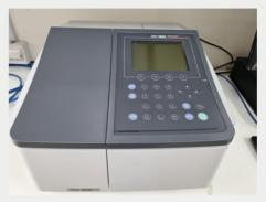
It is an analytical technique that measures the amount oflight that is absorbed by the solution in a cuvetteplaced in the spectrophotometer. Is a widely used technique in many areas of science:
