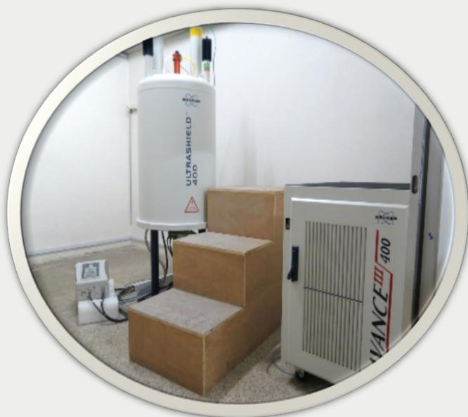
NMR Spectroscopy is a technique used to determine the chemical molecular structure of organic compounds.
