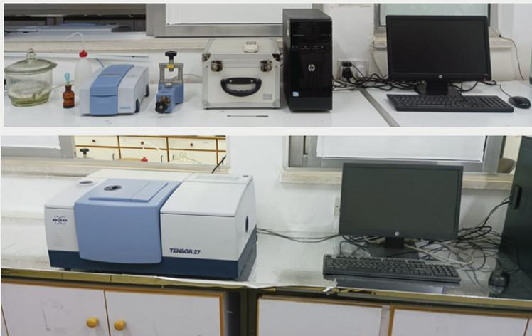
FT-IR is used to obtain the IR spectra of different organic and inorganic chemical compounds. The theory depends on the vibrational modes of chemical bonds in different chemical compounds. The resulted IR spectrum covers the range of  $400\text{cm}^{-1}$  -  $4000\text{cm}^{-1}$ . It reveals the types of chemical bonds present in the chemical compounds and hence reveals the functional groups suspected to be presented in the sample.
