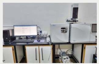
It is an analytical separation technique applicable to gas, liquid, and solid samples (components that are vaporized by heat). Combines two analytical tools to identify compounds and measure the concentration of chemicals found in food, oils, pharmaceuticals, the environment and more.
