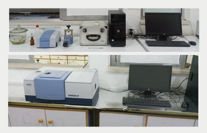
FT-IR is used to obtain the IR spectra of different organic and inorganic chemical compounds. The theory depends on the vibrational modes of chemical bonds in different chemical compounds. The resulted IR spectrum covers the range of 400cm<sup>-1</sup> - 4000cm<sup>-1</sup>. It reveals the types of chemical bonds present in the chemical compounds and hence reveals the functional groups suspected to be presented in the sample.
