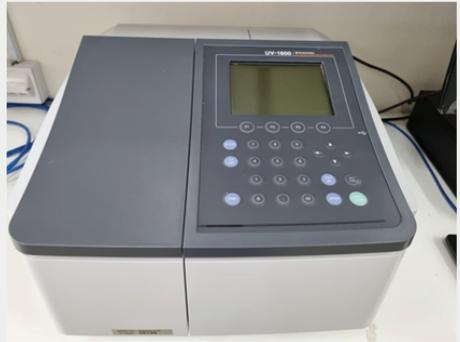
It is an analytical technique that measures the amount of light that is absorbed by the solution in a cuvette placed in the spectrophotometer. It is a widely used technique in many areas of science:
