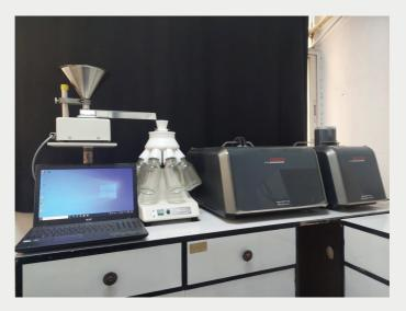
Laser Particle Analyzer (LPA) (Model Analysette 22 MicroTec Plus)
